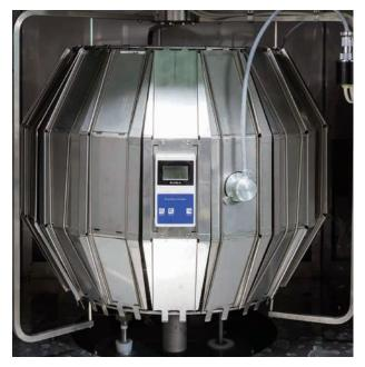
Radiometer on the weather meter (Model SX75)
