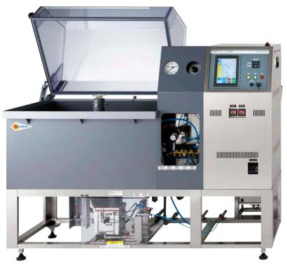
The mist dispersion tower provides uniform distribution of the spray, and it is in conformance with standards such as ISO, JIS and JASO. This is an economical test instrument that performs the test of many specimens and also component parts at the option.
