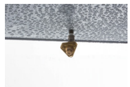
■Water spray test SAE J575 Type A
