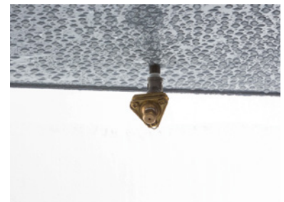
■Water spray test SAE J575 Type A
